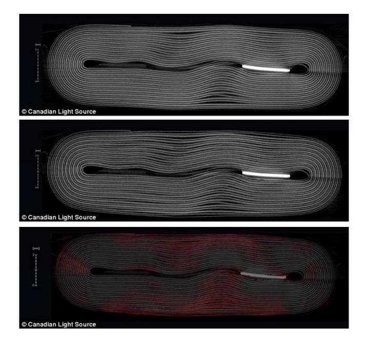
A battery pouch cell (top) before and after (middle) pillowing. In the third image (bottom), the differences between the two states are highlighted in red, where it is clear that most of the change occurs in the flat portion of the battery jellyroll.
