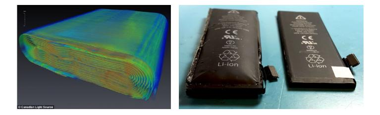
The pillowing effect is the main reason for batteries failing, and in extreme cases can lead to fire.
