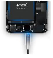
It's quite simple. We detect when the battery is fully charged, and then stop the charging by physically breaking the circuit using a relay. Its like you are unplugging your phone, without having to unplug it.
